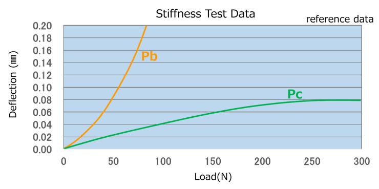
✓ Use as this direction is recommended, since smaller displacement at Pc direction.
