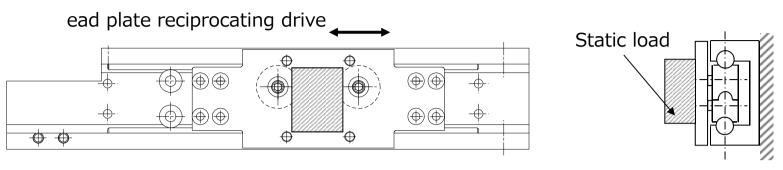
Condition: Normal Temperature, average speed 0.1m/s, load 10kgf, stroke0.26m, 0.36m
